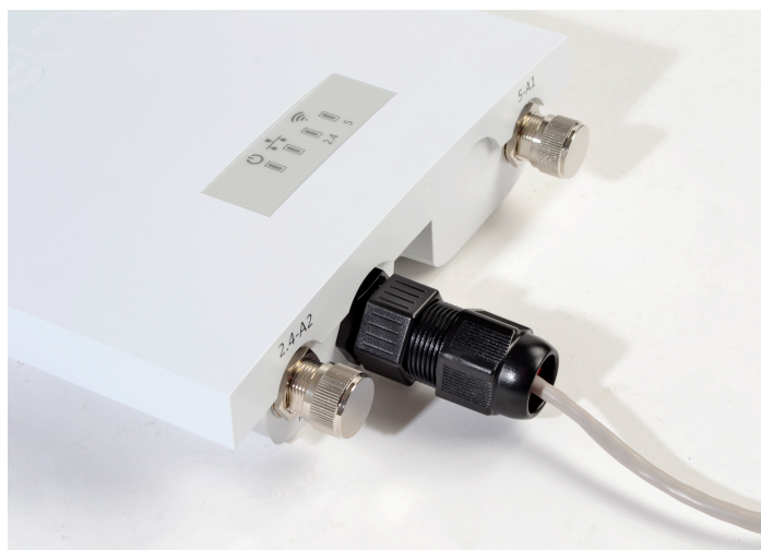
Figure 24 – View of the connected cable to the device network interface
