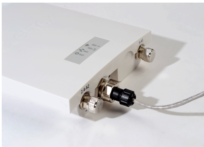
Figure 23 – View of the connected cable to the device network interface
