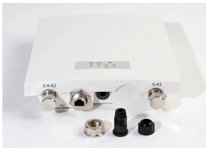
Figure 14 – Hermetically sealed RJ-45 connector of the device and counterpart in disassembled state for hardware versions 1v0, 1v1 and 1v2
